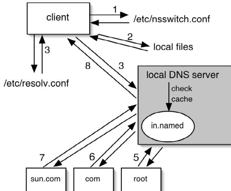
Traffic between the client and its local DNS server is "recursive", insofar that the client will keep on waiting for an answer. In the meanwhile the DNS server may query other DNS servers for the real answer. In technical terms the DNS client is also called the "resolver".
