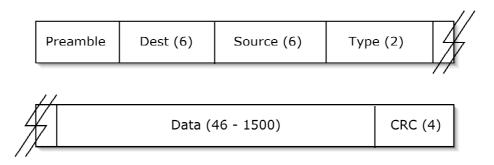
Above you see the layout of an Ethernet frame. Each field has both its name and its size (in bytes) printed in each label. As you can see the overhead in an Ethernet frame consists of 14 bytes in the header and an extra 4 bytes in the form of the Cyclic Redundancy Check. Hence, the minimum frame size is 64 B and the maximum size would be 1518 bytes.
